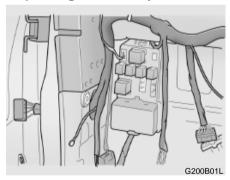
The instrument panel junction box for the lights and other electrical accessories will be found low on the dashboard on the driver's side. Inside instrument panel junction box you will find a list showing the circuits protected by each fuse.
