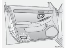
A red light comes on when the door is opened. The purpose of this light is to assist when you get in or out and also to warn passing vehicles.
