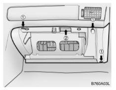
4. Remove the lower crash pad mounting screws (1) and nut (2), and then detach the lower crash pad.
