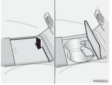
The drink holder is located on the main console for holding cups or cans. The drink holder can be opened by pushing at its top edge.
