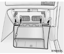
3. Remove the glove box mounting bolts (1) and screws (2) from the glove box assembly, and then detach the glove box assembly.
