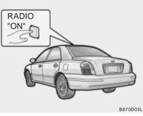
When the radio power switch is turned on while the ignition key is in either the "ON" or "ACC" position, your car will receive both AM and FM broadcast signals through the antenna in the rear window glass. CAUTION:
