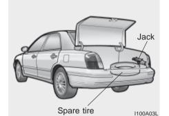
Remove the spare tire and take out the jack and tool bag from the trunk.
