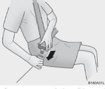
To fasten your seat belt, pull it out of the retractor and insert the metal tab into the buckle. There will be an audible "click" when the tab locks into the buckle.
