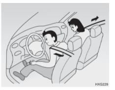
The pre-tensioner seat belt operates in a similar way as an Emergency Locking Retractor (ELR) type of seat belt. When the vehicle stops suddenly, or if the occupant tries to lean forward too quickly, the seat belt retractor will lock into position. However, in certain frontal collisions, the pre-tensioner will activate and pull the seat belt into tighter contact against the occupant's body.
