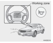
Press the center hub on the steering wheel to sound the horn.
