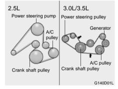
When the air conditioning is being used regularly, the compressor drive belt tension should be checked at least once a month.
