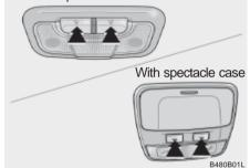
Push in the map light switch to turn the light on or off. This light produces a spot beam for convenient use as a map light at night or as a personal light for the driver and the passenger.
