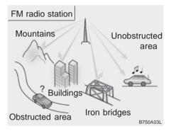
FM broadcasts are transmitted at high frequencies and do not bend to follow the earth's surface. Because of this, FM broadcasts generally begin to fade at short distances from the station. Also, FM signals are easily affected by buildings, mountains, or other obstructions. These can result in certain listening conditions which might lead you to believe a problem exists with your radio. The following conditions are normal and do not indicate radio trouble:
