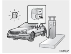
The fuel-filler lid may be opened from inside the vehicle by pushing on the fuel-filler lid opener located on the driver's door.
