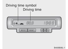
o **DISTANCE TO EMPTY** - This mode indicates the estimated distance to empty from the current fuel in the fuel tank. When the remaining distance is below 50km(30miles), "----" symbol will be displayed with blinking.
