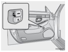
To open the trunk lid without using the key, pull up the lid release lever.
