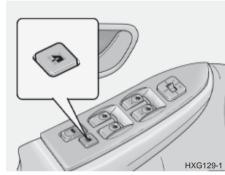
In order to prevent operation of the windows, a window lock switch(2) is provided on the armrest of the driver's door. To disable the power windows, press the window lock switch. To revert to normal operation, press the window lock switch a second time. The power windows can be operated for 30 seconds after the ignition key is turned to the "ACC" or the "LOCK" position. However while the front doors are opened with the key turned to "LOCK" and removed, the power windows cannot be operated.
