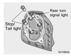
3. To replace the rear combination light (stop/tail light and rear turn signal light), take out it from the bulb holder and install the new bulb. BACK UP LIGHT 1. Remove the trunk lid trim.
