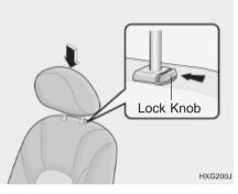
Headrests are designed to help reduce the risk of neck injuries. To raise the headrest, pull it up. To lower it, push it down while pressing the lock knob. If equipped with a horizontally adjustable type of headrest, pull on the top.
