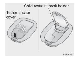
1. Open the tether anchor cover on the rear seat package tray.
