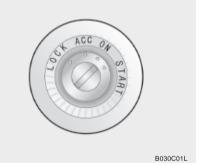
Whenever a door is opened, the ignition switch will be illuminated for your convenience, provided the ignition switch is not in the "ON" position. The light will go off approximately 10 seconds after closing the door or when the ignition switch is turned on.
