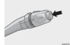
If a single wipe is desired in mist, push the MIST operation switch at the end of the windshield wiper and washer control lever. Adjustable Intermittent Wiper Operation
