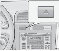
The hazard warning system should be used whenever you find it necessary to stop the car in a hazardous location. When you must make such an emergency stop, always pull off the road as far as possible.
