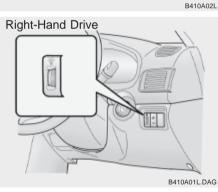
The instrument panel lights can be made brighter or dimmer by turning the instrument panel light control knob.
