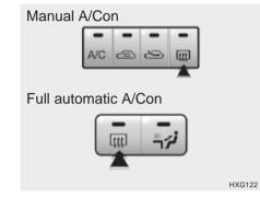
The rear window defroster is turned on by pushing in the switch. At the same time, the rear window defroster indicator light on the switch is turned on. To turn the defroster off, push the switch a second time. The rear window defroster automatically turns itself off after about 20 minutes. To restart the defroster cycle, push in the switch again after it has turned itself off.
