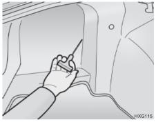
If the fuel filler lid cannot be opened using the remote opener, a manual opener handle is located inside the trunk on the left side. Open the fuel filler lid by pulling on this handle as shown illustration.
