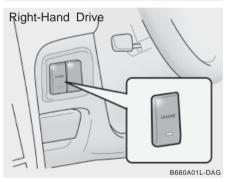
The cruise control system provides automatic speed control for your comfort when driving on freeways, tollroads, or other noncongested high ways. This is designed to function above approximately 40 km/h (25 mph).
