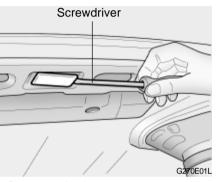
2. Remove the luggage compartment light cover on the rear package tray panel with a blade screwdriver.
