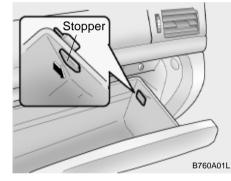
1. Open the glove box. Remove the stoppers on the both sides of the glove box.
