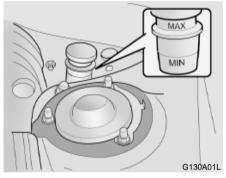
The clutch fluid level in the master cylinder should be checked when performing other under hood services. The system should be checked for leakage at the same time.
