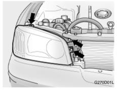
1. Remove the headlight assembly mounting bolts.
