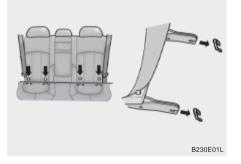
To engage the child restraint seat to the ISOFIX anchor, insert the child restraint seat latch into the ISOFIX anchor. Listen for the audible "click" sound. 2. Connect the tether strap hook to the child restraint hook holder and tighten to secure the seat. Refer to "Securing a Child Restraint System With Tether Anchorage System" on page 1-26.
