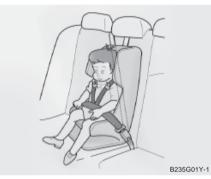
Use the center seat belt for the rear to secure the child restraint system as illustrated. After installation of the child restraint system, rock the child seat back and forth, and side to side to ensure that it is properly secured by the seat belt.
