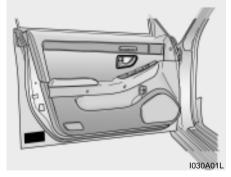
The tire label located on the driver's door edge gives the tire pressures recommended for your car.
