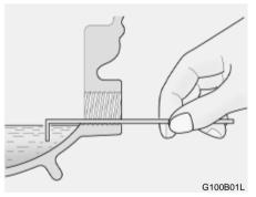
Park the car on level ground with the engine off.
