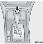
The highly efficient Hyundai automatic transaxle has four/five forward speeds and one reverse speed. The individual speeds are selected automatically, depending on the position of the speed selector lever. The selector lever has 2 gates; the main gate and the manual gate.
