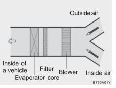
The air filter is located in front of the evaporator unit behind the glove box. It operates to decrease pollutants from entering the car and to filter the air. To replace the air filter, refer to the page 6-18.
