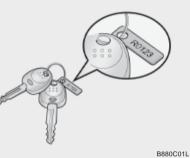
The vehicle key number is recorded upon a metal tag attached to the keys when the vehicle is first delivered to you.
