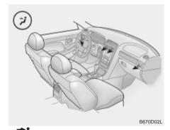
**Face-Level** When selecting the "Face" mode, the indicator light will come on, causing air to be discharged through the face level vents.
