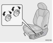
To raise or lower the front part of the seat cushion, turn the front knob forward or rearward. To raise or lower the rear part of the seat cushion, turn the rear knob forward or rearward.
