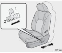
Pull the control knob forward or backward to move the seat forward or backward to the desired position. Release the knob and then the seat will remain at that position.
