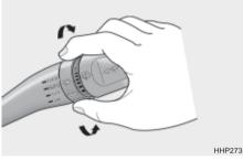
To use the intermittent wiper feature, place the wiper switch in the "INT" position. With the switch in this position, the interval between wipes can be varied from approximately 1 to 18 seconds by turning the interval adjuster barrel. This is also varied automatically depending on your road speed.
