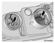
4. Disconnect the power cord from the bulb base in the back of the headlight.
