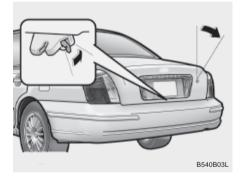
If the trunk lid lock knob (located near the latch) is in the "LOCK" position when the trunk lid is closed, it will not be possible to open the trunk lid by using the remote release. In this instance, use the master key to unlock and open the trunk lid.
