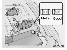
A fusible link will melt if the electrical circuits from the battery are ever overloaded, thus preventing damage to the entire wiring harness. (This could be caused by a short in the system drawing too much current.) If this ever happens, have a Hyundai dealer determine the cause, repair the system and replace the fusible link. The fusible links are located in a under hood junction box for easy inspection.
