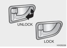
To lock the doors from the inside, simply close the door and push the lock switch to the "LOCK" position. When this is done, neither the outside nor the inside door handle can be used.
