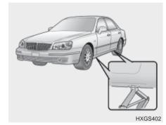
The base of the jack should be placed on firm, level ground. The jack should be positioned as shown in the drawing. 5. Raising the Car
