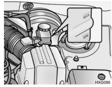
The fluid level in the brake fluid reservoir should be checked periodically. The level should be between the "MIN" and "MAX" marks on the side of the reservoir. If the level is at or below the "MIN" mark, carefully add fluid to bring it up to "MAX". Do not overfill. G120E02A-AAT Adding Brake Fluid
