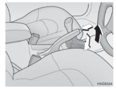
Always engage the parking brake before leaving the car. This also turns on the parking brake indicator light when the key is in the "ON" or "START" position. Before driving away, be sure that the parking brake is fully released and the indicator light is off.
