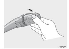
To use the windshield washer, pull the wiper/washer lever toward the steering wheel. When the washer lever is operated, the wipers automatically make two passes across the windshield. The washer continues to operate until the lever is released.
