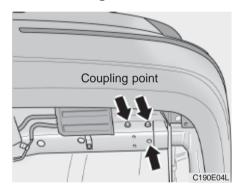
5. The maximum permissible overhang of the coupling point : 1,230 mm.
