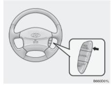
The vehicle will automatically resume the speed set prior to cancellation when you push the control switch "RESUME (ACCEL)" (above 40 km/h).
