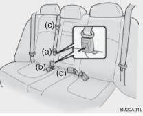
1. Before fastening the rear seat center belt, confirm the metal tab (a) and buckle (b) are latched together.
