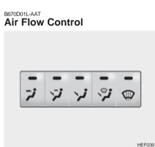
This is used to direct the flow of air. Air can be directed to the floor, dashboard outlets, or windshield. Five symbols are used to represent Face, Bi-Level, Floor, Floor-Defrost and Defrost air position.
