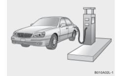
Unleaded gasoline with a Pump Octane Rating of 87 (Research Octane Number 91) or higher must be used in Hyundai vehicle. If leaded gasoline is used, it will cause the catalytic converter to become ineffective and the emission control system to malfunction.
