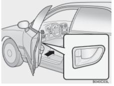
The doors can be locked without a key. To lock the doors, first push the inside lock switch to the "LOCK" position, so that the red mark on the switch is not visible, then closed the door.
