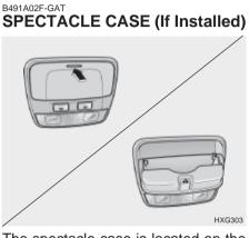
The spectacle case is located on the front overhead console. Push the end of the cover to open the spectacle case.
