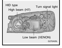
o You can replace the high beam (H1 or H7) and front turn signal light. The replacement instruction is same with the general type's one. But you must not replace or inspect the low beam (XENON bulb). It has a danger of an electric shock. If the low beam (XENON bulb) is not working, have your vehicle inspected by your Hyundai Dealer.
