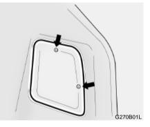
2. Remove the cover on the inside of rear luggage trim by unscrewing the screws.
