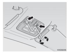
2. Remove the front overhead light and switch panel, using a phillips screwdriver.
