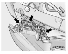
2. Disconnect the power cord from the bulb base in the back of the headlight.
