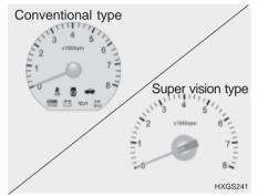
The tachometer registers the speed of your engine in revolutions per minute (rpm). It is useful to help you shift at the appropriate engine speed to avoid lugging or over-revving the engine.
