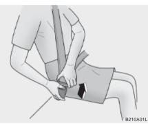
The seat belt is released by pressing the release button in the locking buckle. When it is released, the belt should automatically draw back into the retractor.
