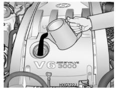
If the oil level is close to or below the "L" mark, add oil until it reaches the "F" mark. To add oil:
