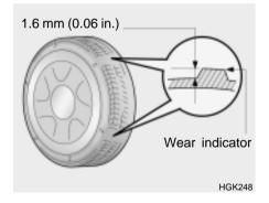
The original tires on your car have tread wear indicators. The tread wear indicators appear when the tread depth is 1.6 mm (0.06 in.). The tire should be replaced when these appear as a solid bar across two or more grooves of the tread. Always replace your tires with those of the recommended size. If you change wheels, the new wheel's rim width and offset must meet Hyundai specifications.
