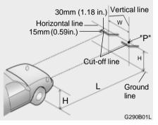
If the vehicle has had front body repair and the headlight assembly has been replaced, the headlight aiming should be checked using an aiming screen as shown in the illustration. Turn on the headlight switch. (Low Beam Position)
