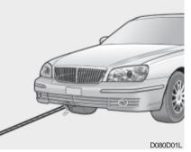
For emergency towing when no commercial tow vehicle is available, attach a tow cable, chain or strap to one of the tie-down hooks under the front of your car. Do not attempt to tow your vehicle in this manner on any unpaved surface. This could result in serious damage to your car.
