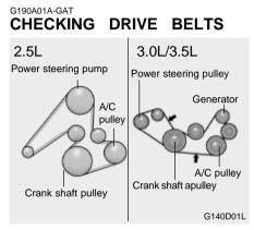
Drive belts should be checked periodically for proper tension and adjusted if necessary. At the same time, belts should be examined for cracks, wear, fraying or other evidence of deterioration and replaced if necessary.
