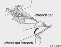
After inserting a wrench bar into the wheel nut wrench, install the wrench bar into the jack as shown in the drawing. To raise the vehicle, turn the wheel nut wrench clockwise. As the jack begins to raise the vehicle, double check that it is properly positioned and will not slip. If the jack is on soft ground or sand, place a board, brick, flat stone or other object under the base of the jack to keep it from sinking.
