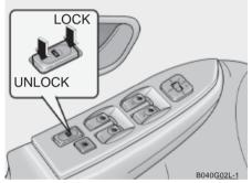
The central door locking switch is located on the driver's arm rest. It is operated by depressing the door lock switch. If any door is open when the switch is depressed, the door will remain locked when closed.
