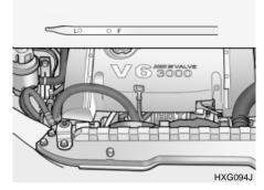
Before checking the oil, warm up the engine to the normal operating temperature and be sure your car is parked on level ground. Turn the engine off.
