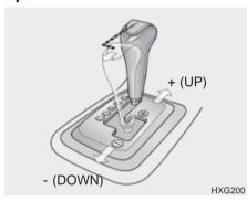
Whether the vehicle is stationary or in motion, sports mode is selected by pushing the selector lever from the "D" position into the manual gate. To return to "D" range operation, push the selector lever back into the main gate. In sports mode, moving the selector lever backwards and forwards can make gearshifts rapidly simply. In contrast to a manual transaxle, the sports mode allows gearshifts with the acceleator pedal depressed.
