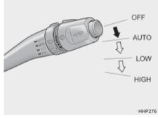
When the windshield wiper switch is placed in the "AUTO" position, the rain sensor located on the upper end of windshield glass senses the amount of rainfall and controls for the appropriate length of the intervals between wipes appropriately.
