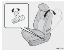
Rotate the upper portion of the control knob forward or backward to recline the seatback to the desired position. Release the control knob and then the seatback will remain in that position. WARNING:
