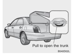
Your vehicle is equipped with a glowin-the dark emergency trunk release lever located inside the trunk. It will glow after the trunk is closed. When pulled, this lever will release the trunk latch mechanism and open the trunk.
