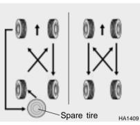
Tires should be rotated every 10,000 km (6,000 miles). If you notice that tires are wearing unevenly between rotations, have the car checked by a Hyundai dealer so the cause may be corrected.
