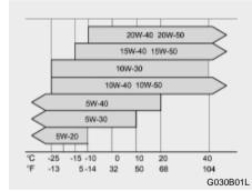
SH, SG or SG/CD (API) multi-grade and fuel efficient oil is recommended.
