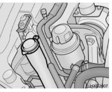
The washer fluid reservoir supplies fluid to the windshield washer system.
