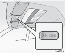
The sunroof can be electrically opened or closed with the ignition key in the "ON" position. To open or to close, press and hold the button located in the front of the roof panel. Release the button when the sunroof reaches the desired position.
