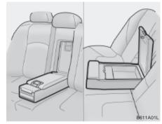
This arm rest is located in the center of the rear seat back with box.
