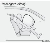
After complete inflation, the airbag immediately starts deflating, enabling the driver to maintain forward visibility.
