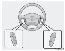
The steering wheel audio remote control switch is installed to promote safe driving. However, do not operate audio remote control switches simultaneously.
