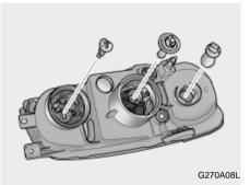
9. To replace the front turn signal light bulb, take out it from the bulb holder and install the new bulb.
