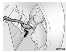
3. Take out front fog light from the bulb holder by turning it counter-clockwise.
