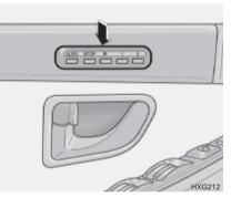
Your vehicle is equipped with I.M.S on the left side of driver's door. After adjusting the position of the driver's seat, outside rearview mirrors and steering wheel column (if installed the steering wheel electric tilt and telescopic), use the I.M.S to memorize them. Two different driving position profiles can be entered in the I.M.S. If you turn the ignition key to the "ON" position, the memorized position is adjusted automatically.
