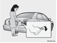
To open the trunk lid, insert the key and turn it clockwise to unlock. The trunk compartment light illuminates when the trunk lid is opened.
