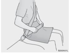
You should place the belt as low as possible on your hips, not on your waist. If the belt is located too high on your body, you could slide under it in case of accident or a sudden stop. This could result of death, serious injury or property damage. Both arms should not be under or over the belt. Rather, one should be over and the other under, as shown in the illustration.
