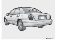
In addition to the lower-mounted rear stoplights on either side of the car, the high mounted rear stoplight in the center of the rear window also lights when the brakes are applied.
