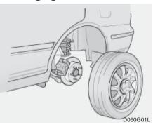
Loosen the wheel nuts and remove them with your fingers. Slide the wheel off the studs and lay it flat so it cannot roll away. To put the wheel on the hub, pick up the spare tire, line up the holes
