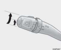
To operate the headlights, turn the barrel on the end of the multi-function switch. The first position turns on the parking lights, sidelights, tail lights and instrument panel lights. The second position turns on the headlights.
