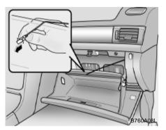
2. Lower the glove box down completely after taking out the damper strap from the hole.
