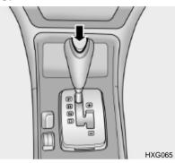
Park the car on level ground with the parking brake engaged. When the transaxle fluid level is checked, the transaxle fluid should be at normal operating temperature and the engine idling.
