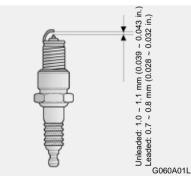
Your engine was originally equipped with platinum-tipped spark plugs. (If installed)
