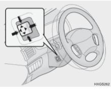
To adjust the desired position of the steering wheel, operate the adjusting switch on the left side of the steering wheel.
