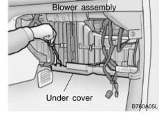
6. Remove the under cover from the blower assembly with pushing the cover toward the floor.
