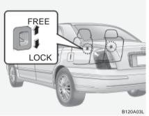
If the rear seatback lock lever (located on the backside of the rear seatback) is in the "LOCK" position when the rear seatbacks are closed, it will not be possible to fold the rear seatback by using the release lock lever. In this instance, move the lock lever to the "FREE" position and fold the rear seatback. The rear seatback lock lever is designed to provide protection from unauthorized entry into the trunk.
