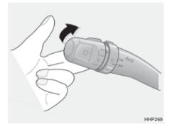
To flash the headlights, pull the switch lever toward you, then release it. The headlights can be flashed even though the headlight switch is in the "OFF" position.
