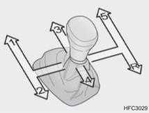
Your Hyundai's manual transaxle has a conventional shift pattern. This shift pattern is imprinted on the shift knob. The transaxle is fully synchronized in all forward gears so shifting to either a higher or a lower gear is easily accomplished.
