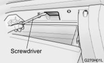
2. Remove the glove box illuminated light cover with a blade screwdriver.
