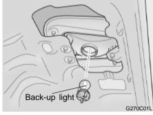
2. To replace the back-up light, take out it from the bulb holder and install the new bulb.
