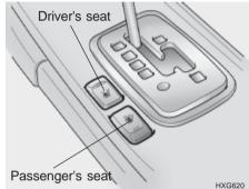
The seat warmer is provided to warm the front seats during cold weather. With the ignition key in the "ON" position, push either of the switches to warm the driver's seat or the passenger's seat.
