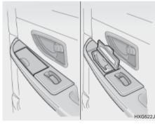
The rear ashtray may be opened by pulling it up by its top edge. To remove the ashtray to empty or clean it, lift it up slightly and pull it all the way out.
