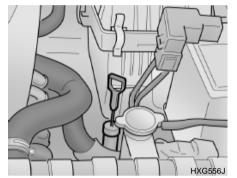
While the engine is idling, apply the brakes and move the gear selector lever from "P" to each of its other positions -- "R", "N", "D" -- and then return to "N". With the engine still idling:
