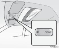
The sunroof can be tilted and closed with the ignition key in the "ON" position. Release the button when the sunroof reaches the desired position.
