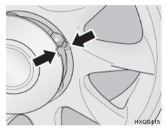
4. Reinstall the wheel cap by fitting the boss of the wheel cap in the groove of the wheel, hitting the center of the wheel cap with hand.
