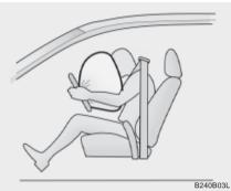
The airbag modules are located both in the center of the steering wheel and in the front passenger's panel above the glove box. When the SRSCM detects a considerable impact to the front of the vehicle, it will automatically deploy the airbags.
