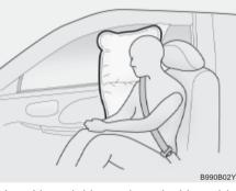
Your Hyundai is equipped with a side airbag in each front seat. The purpose of the airbag is to provide the vehicle's driver and/or the front passenger with additional protection than that offered by the seatbelt alone. The side impact airbags are designed to deploy only during certain side impact collisions, depending on the crash severity, angle, speed and point of impact. The air bags are not designed to deploy in all side impact situations.
