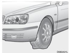
The procedure described on the following pages can be used to rotate tires as well as to change a flat tire. When preparing to change a flat tire, check to be sure the gear selector lever is in "P" (automatic) or reverse gear (manual transaxle) and that the parking brake is set, then: D060K01FC-GAT Wheel Cap (If installed)
