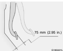
You need a helper to check the brake pedal clearance. With the engine running, have your helper press down on the brake pedal several times and then hold it down with a force of about 490 N (50 Kg, 110 lbs). The brake pedal clearance is the distance from the top surface of the brake pedal to the asphalt sheeting under the floor mat.
